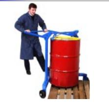
To lower the drum to floor or onto a pallet, the operator pushes down and uses the two hand operated releases and allows the handle to rise. The length of the handle provides leverage to manage the descent of the drum gently.
