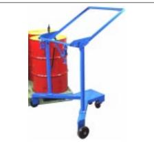
The handle of the Drum-Spotter is conveniently held up by a gas spring. The ratchets stop the handle in position for the operator to take hold and use it. These ratchets also hold the weight of the drum.
