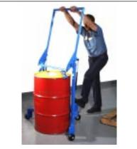
The forged steel hooks release their hold after the drum settles on the floor or pallet deck. This picture also shows the starting position for lifting a drum from the floor.
