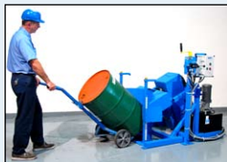
Load drum at floor level with drum truck or crane
