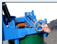
1. Manually secure clamp to grip drum
