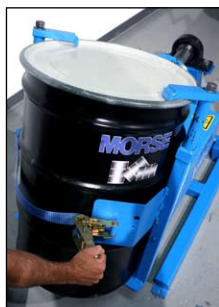
Secure drum with web strap and 2 top clamps
