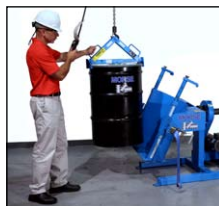
Load with hoist or crane
