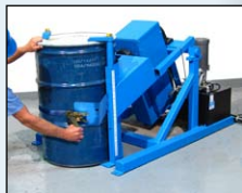
Secure drum with web strap and two top clamps
