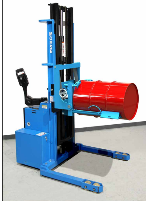
3. Tilt drum to horizontal and transport to racking location
