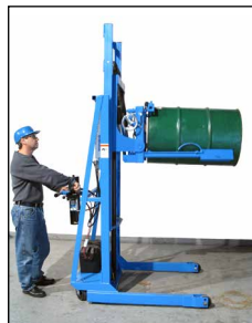
4. Manually release clamp. Raise drum to place in rack.
