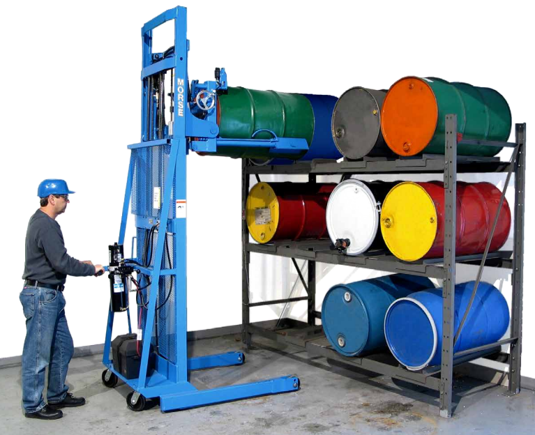
3. Tilt drum to horizontal and transport to racking location
